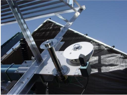
Fig. 8: Solar radiation measurement and tracking sensors.
