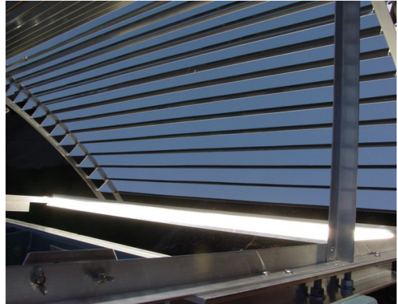
Fig. 9: A 6 ft. long focal line created by the array of slats.
