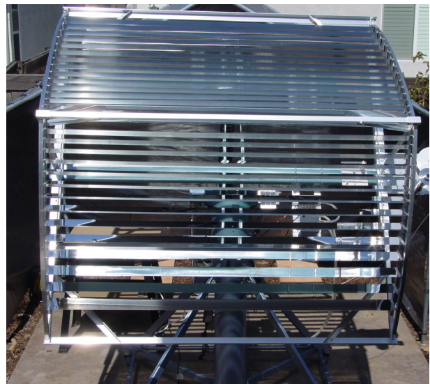
Fig. 3: Experimental slat-array CPV.
