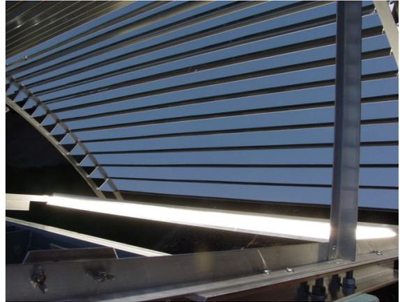
Fig. 9: A 6 ft. long focal line created by the array of slats.
