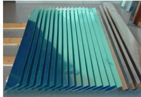
Fig. 2: A sample batch of slat reflectors.
