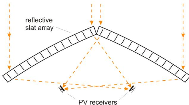
Fig. 1: A conceptual design of slat-array CPV.
