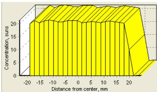
Fig. 5: The positive effect of a secondary reflector on flux distribution.
