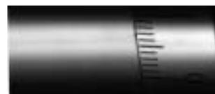
Fig. 10: Focal image of the concentrator focal spot. The scale is graduated in 1-mm increments.
