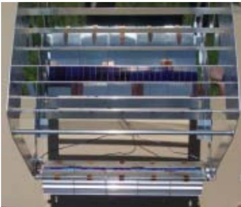
Fig. 1: Top view of the experimental slat-array CPV
