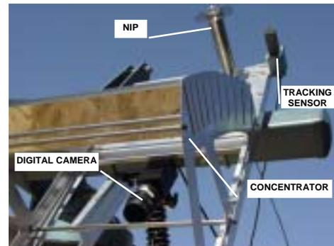
Fig. 5: The prototype concentrator under testing
