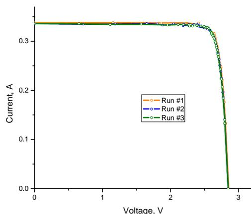
Fig. 8: Experimental I-V curves for the single-cell receiver
