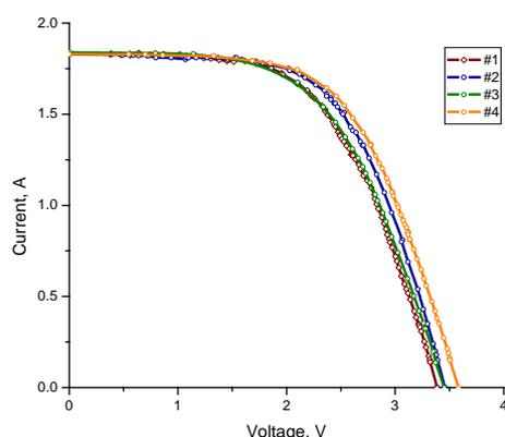
Fig. 6: Measured I-V curves for different receiver modules
