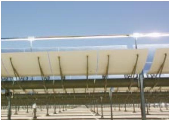
Above: The new Solel UVAC trough receiver tubes under test at SEGS VI in California by KJC Operating Co. and NREL.
