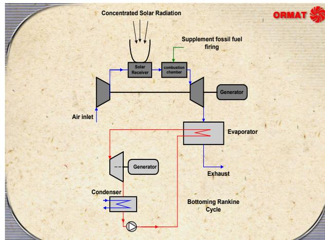
Fig. 3. Combined Cycle Power generation System
