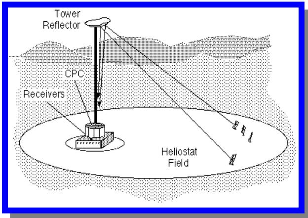
Figure 2 – High Concentration Beam Down Configuration
