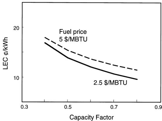
Fig. 10. Levelized energy cost for the 600 kW<sub>e</sub> SCOT/CC plant as a function of capacity factor and fuel price.
