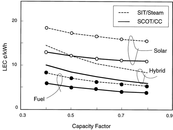
Fig. 8. Levelized energy cost of the solar-derived (open circles), fuel-derived (solid circles) and overall electricity, as a function of plant capacity factor. Solid lines: 34 MW<sub>e</sub> SCOT/CC plant; dashed lines: SIT/steam plant. Fuel price of 2.5 \$/MBTU and FCR of 14% were assumed.
