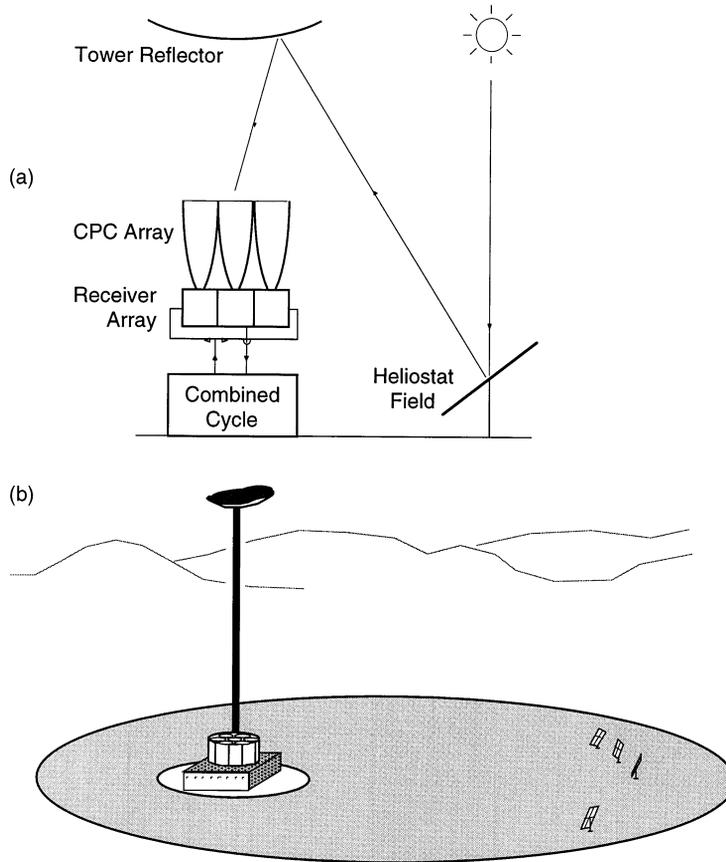
Fig. 2. The new concept of a solar-driven CC plant. (a) plant schematic; (b) artist's view, approximately to scale, of the 34 MW<sub>e</sub> plant.
