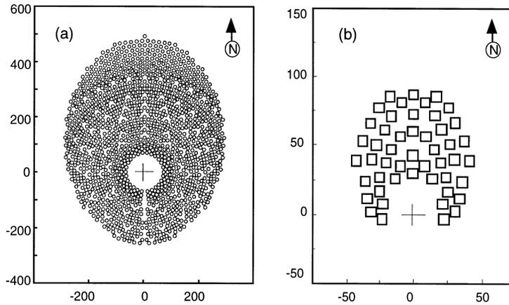
Fig. 5. Heliostat field layout for the two example SCOT/CC plants: (a) 34 MW<sub>e</sub>; (b) 600 kW<sub>e</sub>. Coordinate grid is in meters. Heliostats are 95 m<sup>2</sup> in (a) and 57 m<sup>2</sup> in (b); see Table 1 for details.
