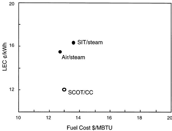
Fig. 9. Solar vs fuel LEC parity points at capacity factor of 0.6, for SCOT/CC, SIT/steam and air/steam plants.
