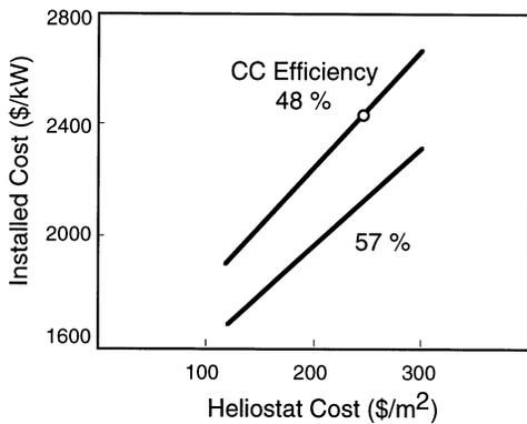
Fig. 6. Effect of heliostat cost and power conversion efficiency on installed cost of the 34 MW<sub>e</sub> SCOT/CC plant. Circle: design point for the present study.
