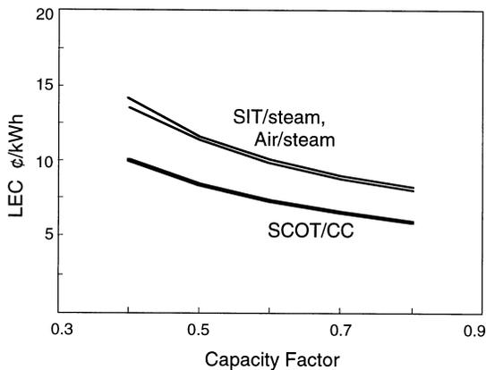
Fig. 7. Levelized energy cost of the 34 MW<sub>e</sub> SCOT/CC, and 30 MW<sub>e</sub> SIT/steam and air/steam plants, as a function of capacity factor in hybrid solar/fossil mode.
