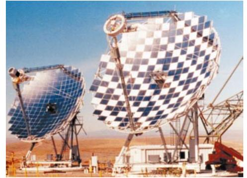
*Component development and testing at Sandia National Laboratories and the National Renewable Energy Laboratory have led to improved and validated optical materials, mirror facets, concentrator structures, receivers, and control systems for all CSP technologies.*
