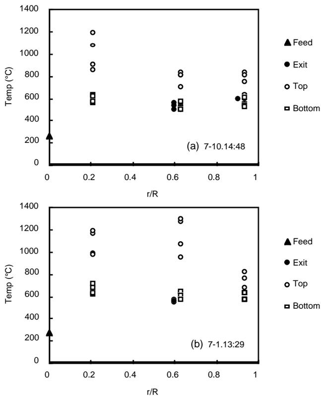
Figure 12. Temperature distribution in Foam and Honeycomb absorbers. O=6 m; L=100 mm. (a) Foam,  $I_n=775 \text{ W/m}^2$ ,  $\dot{m}=7.36 \cdot 10^{-3} \text{ kg/s}$ . (b) Honeycomb,  $I_n=821 \text{ W/m}^2$ ,  $\dot{m}=7.33 \cdot 10^{-3} \text{ kg/s}$ .
