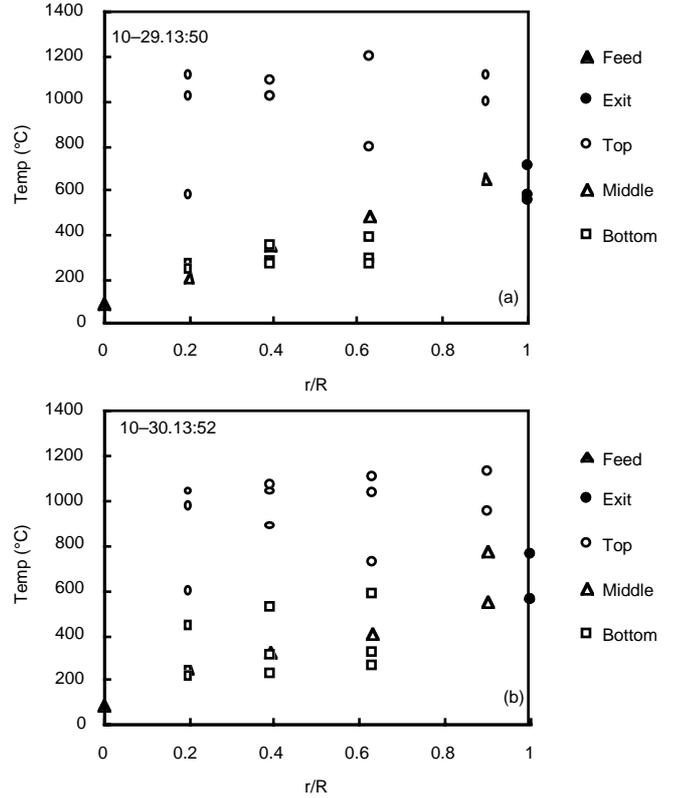
Figure 8. Temperature distributions for *Porcupine* #2.  $L=30$  mm; (a) Inlet configuration H1;  $I_n=660$  W/m<sup>2</sup>,  $\dot{m}=6.16 \cdot 10^{-3}$  kg/s,  $O=4$  m. (b) Inlet configuration H2;  $I_n=675$  W/m<sup>2</sup>,  $\dot{m}=6.18 \cdot 10^{-3}$  kg/s,  $O=4$  m.
