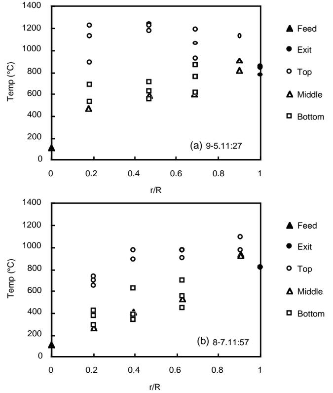
Figure 10. Temperature distributions in *Porcupine* #4 with inlet H4,  $O=6$  m. (a)  $L=30$  mm,  $I_n=784$   $\text{W/m}^2$ ,  $\dot{m}=11.7 \cdot 10^{-3}$  kg/s. (b)  $L=100$  mm,  $I_n=815$   $\text{W/m}^2$ ,  $\dot{m}=7.36 \cdot 10^{-3}$  kg/s.
