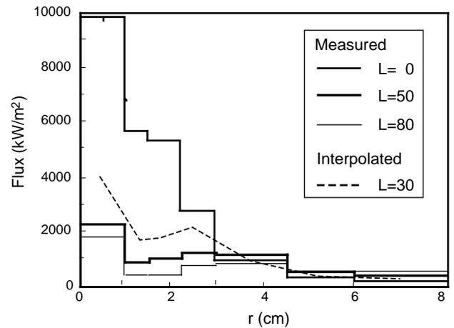
Figure 4. Distribution of local irradiation flux as a function of radius and distance behind the focal plane (after Rosin et al., 1986); Furnace door opening is  $O=6$  m. Flux values are normalized for incident radiation of  $800 \text{ W/m}^2$ .
