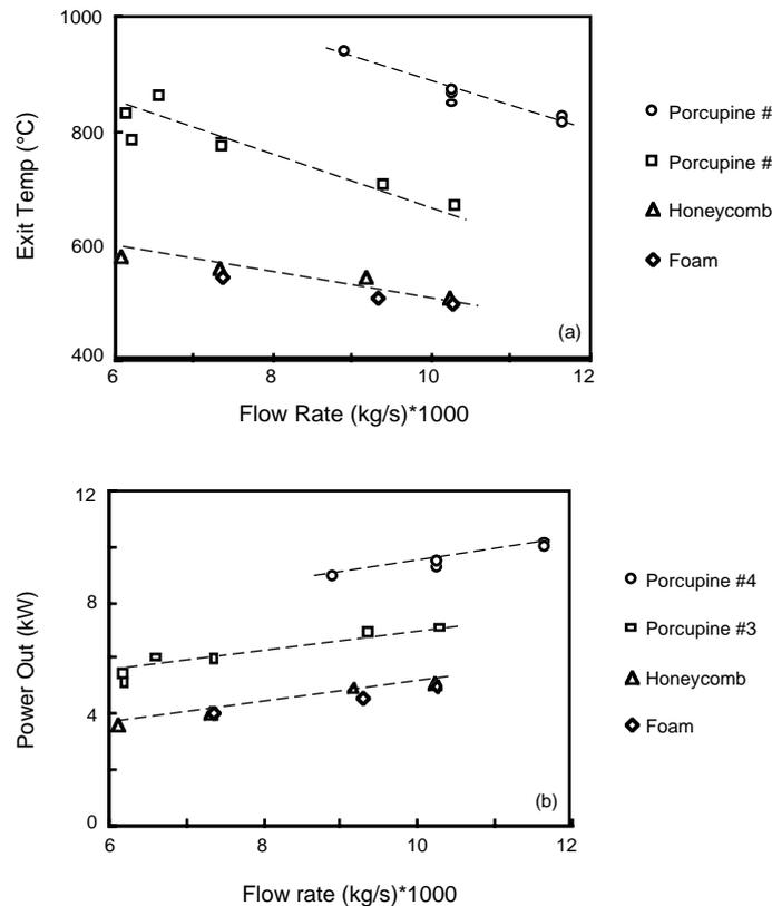
Figure 13. Comparison of (a) exit gas temperature and (b) power output of the Honeycomb, Foam and two *Porcupine* absorbers. Only tests where absorber temperature approached the maximum allowed limit are included.
