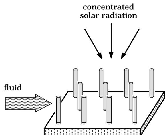
Figure 1. The *Porcupine* Volumetric solar absorber concept.
