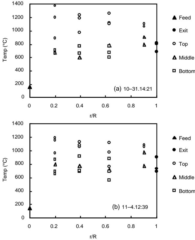
Figure 9. Temperature distributions for *Porcupine* #3.  $L=30$  mm; (a) Inlet configuration H2;  $I_n=674$   $\text{W/m}^2$ ,  $\dot{m}=6.18 \cdot 10^{-3}$  kg/s,  $O=6$  m. (b) Inlet configuration H3;  $I_n=730$   $\text{W/m}^2$ ,  $\dot{m}=7.38 \cdot 10^{-3}$  kg/s,  $O=6$  m.
