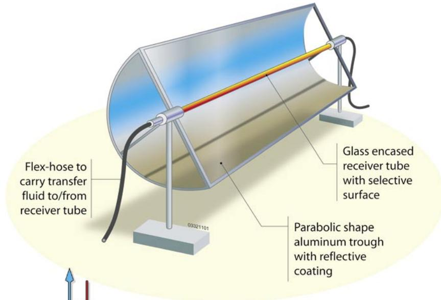
Figure 1: Parabolic trough collector
