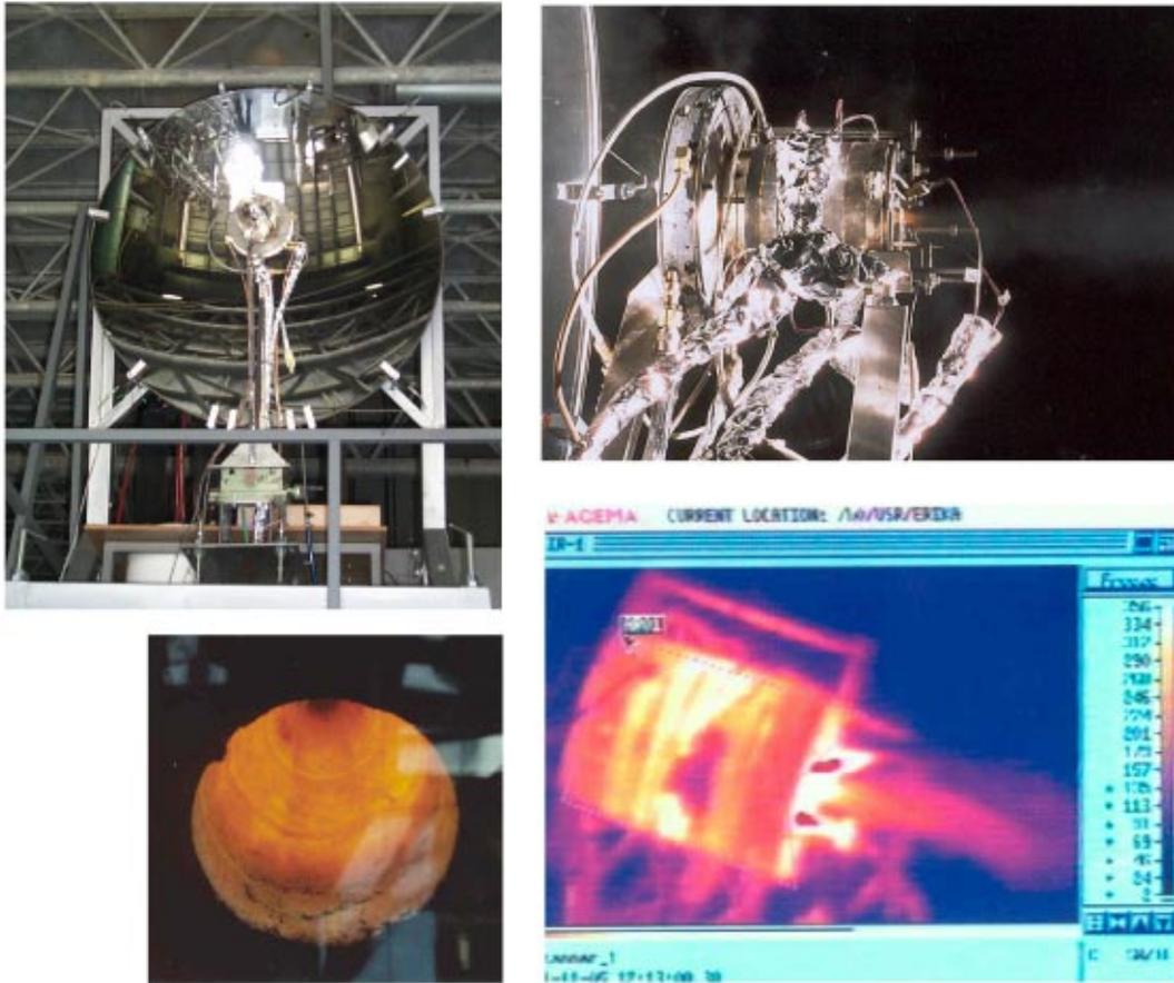
Top left: The test set-up, located 30 m above the heliostat field, consists of a secondary 1.5 m parabolic dish and the particle receiver. Right: The solar particle receiver in operation. The exhaust gas and particle plume is visible on the right.
