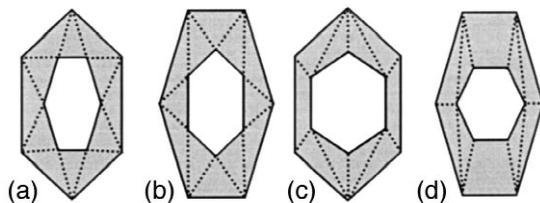
Fig. 6. Various types of interconnections between non-regular hexagonal apertures by plane facets. (a) V-type to H-type, (b) H-type to V-type, (c) V-Type to V-type, (d) H-type to H-type. The interconnections between the non-parallel sides by triangular facets in (c) and (d) are not unique.
