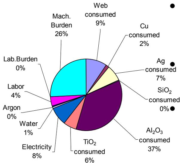
**Projected breakdown of costs for super thin glass reflector (total cost = \$10.14/m<sup>2</sup>)**
