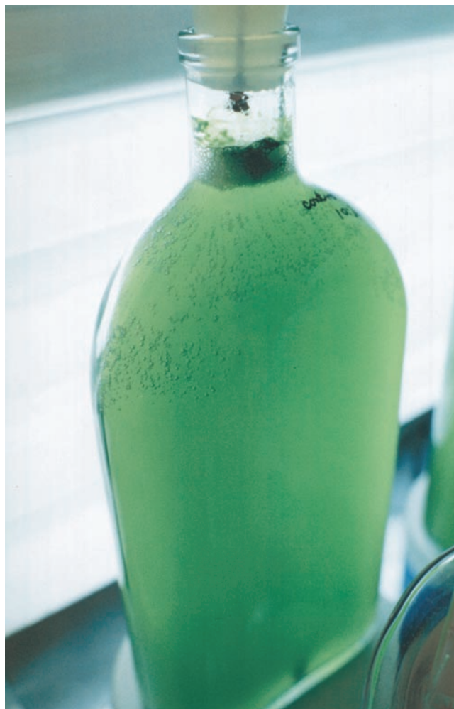
Figure 1. A hydrogen-producing C. reinhardtii culture. Hydrogen bubbles emanate toward the surface of the liquid medium. The gas is drained through a syringe (inserted in the middle of the silicone stopper) and, through teflon tubing, is collected in an inverted burette and measured by the method of water displacement. Photograph courtesy of Michael Barnes (Office of the President, University of California, Oakland).
