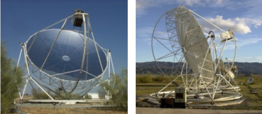
Figure 8: Front and side view of the EURODISH system
