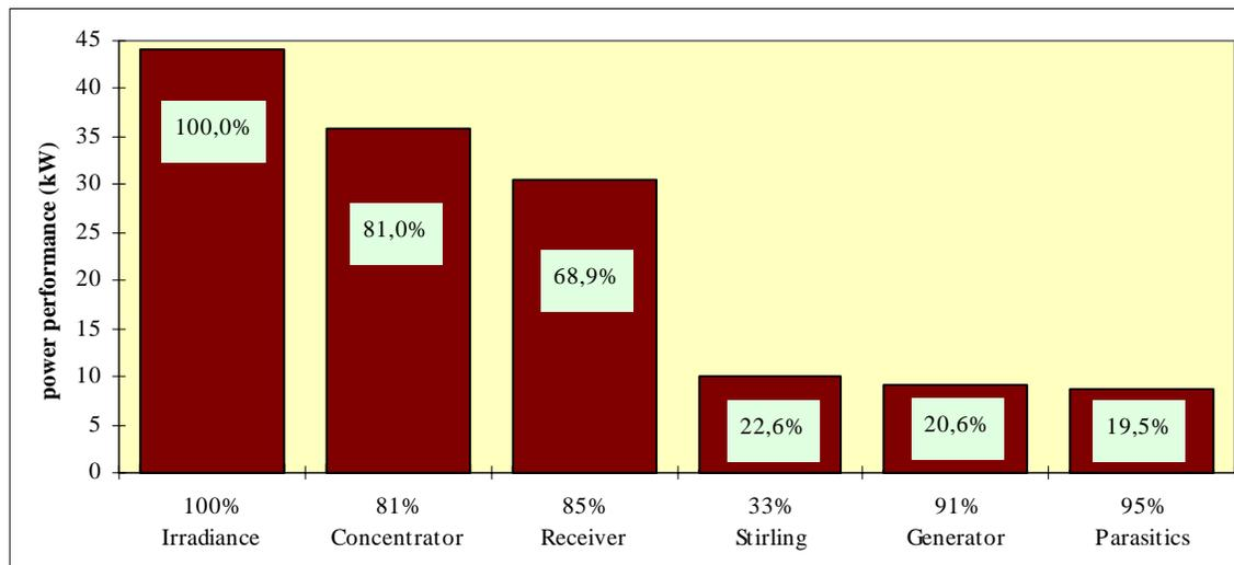
Figure 2: Performance of subcomponents of DISTAL I at 850 W/m<sup>2</sup>
