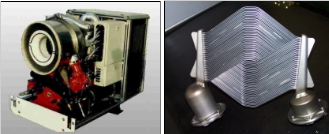
Figure 9: SOLO V161 Stirling engine (left) and metallic, tubular solar receiver (right)
