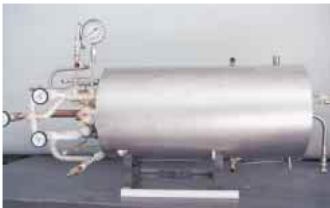
This innovative fuel processor by Northwest Power Systems can convert a number of fuels into high purity hydrogen to power a fuel cell stack.
