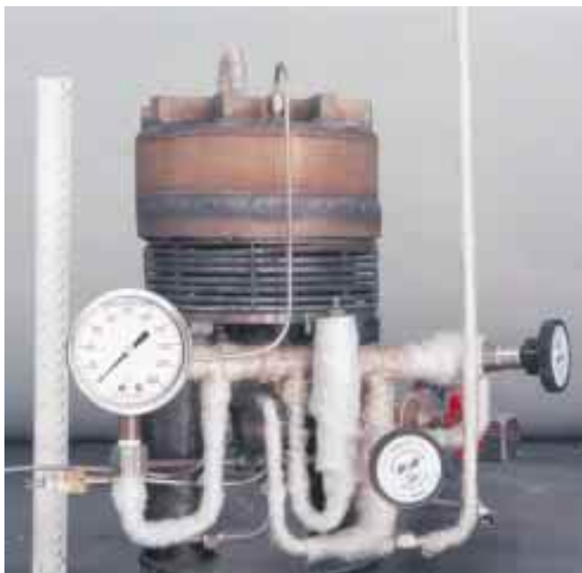
This remarkably compact fuel processor by Northwest Power Systems can deliver enough high purity hydrogen to power a 1 KW fuel cell.
