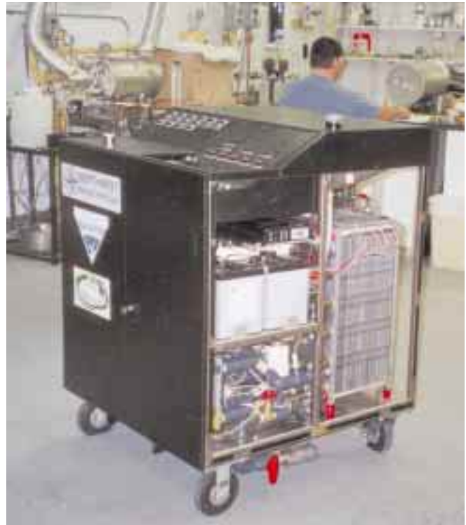
The Northwest Power Systems 5 KW mobile demonstration fuel cell system. Note the fuel cell located on the right side of the unit.
