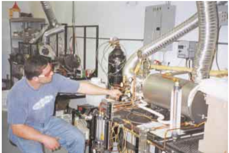
A technician tests a fuel processor that runs on kerosene and produces up to 50 liters per minute of hydrogen containing about 2 ppm of CO.
