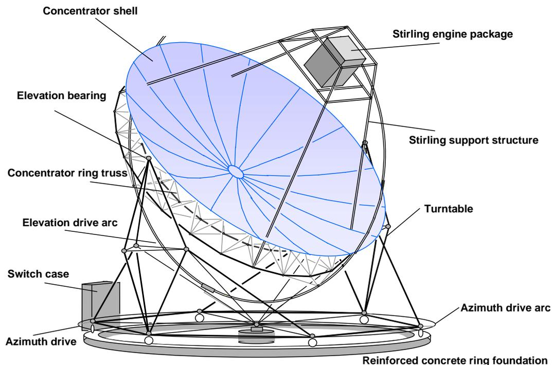
**Dish-Stirling Systems** transfer concentrated solar radiation with high efficiencies into electrical energy. Essentially the system consists of the following components:
