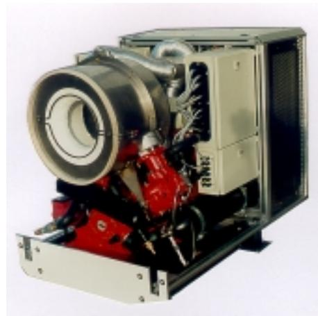
Schlaich Bergermann und Partner (SBP) together with SOLO developed the V160/V161 Stirling engine seen in the pictures. This is currently the most reliable and most advanced Stirling engine available (Picture with solar-only receiver).
