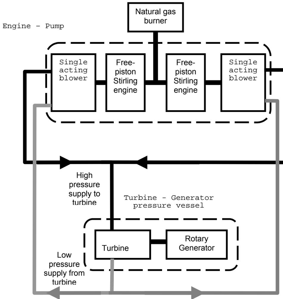
Figure 1. System Schematic
