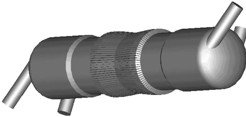
Figure 6. Opposed engine / blower pair with burner
