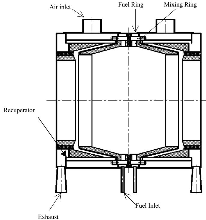
Figure 3. Burner layout
