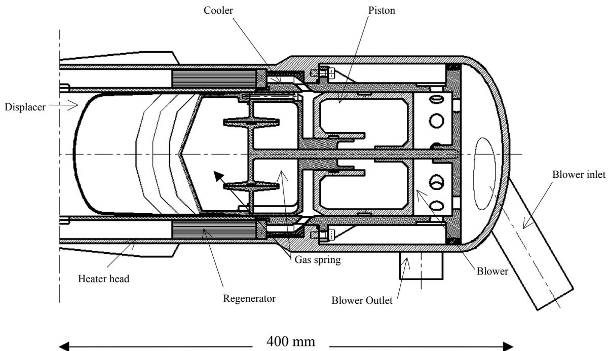
Figure 2. Single engine and blower (from opposed pair)
